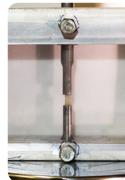
Measuring compressive strength with Instron 5866 Universal tester
